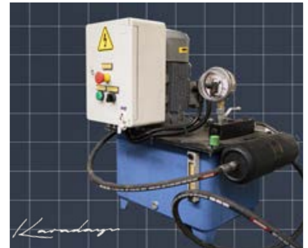
Hydraulic unit that provides control of roller gap
