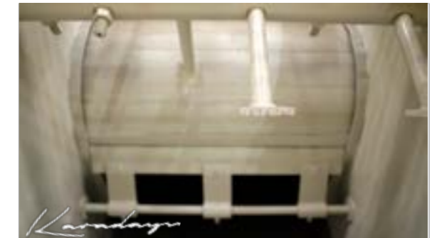
Paddle shaft with cranked and serrated blades for crumbly or preprocessed materials, made from HARDOX 600.
