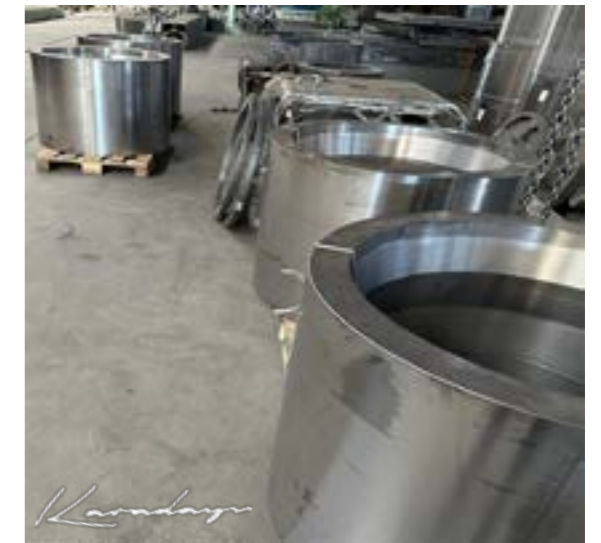
Roller material is spheroidal casting, and hardness is 46 - 50 HRC
